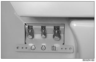
Put a container capable of holding at least 12.3 liter (13 U.S. quarts) below engine oil drain. Remove cap and drain oil into container. Install cap after oil has drained.
