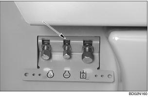
Put a container capable of holding at least 22.7 liter (6.0 gallon) below radiator drain. Remove radiator cap. Remove cap and drain coolant into container. Install cap after coolant has drained. Install radiator cap.
