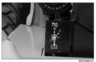
The master disconnect is located under the hood on the left read side of the machine. Raise the hood put master disconnect switch in OFF position. Remove both battery covers and disconnect batteries from the machine.
